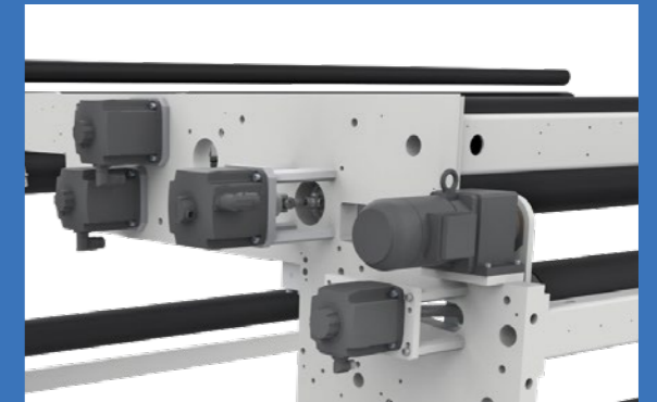
Individual roll drives For sensitive films like high barrier, capacitor or BOPE films
